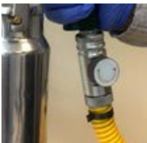
Product regulator by roulette with flow indicator
