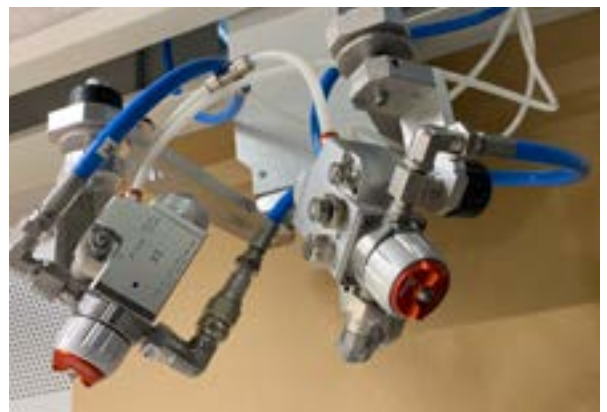
Installation of V7 mix automatic guns in robot version
