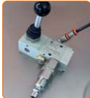
Manual operation valve
